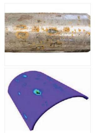
The Laser Mapper makes laser corrosion mapping practical. It works on smooth, shiny and dull or rough surfaces without any special surface preparation. The Laser Mapper is capable of scanning at high resolutions at up to 30 inches per second
